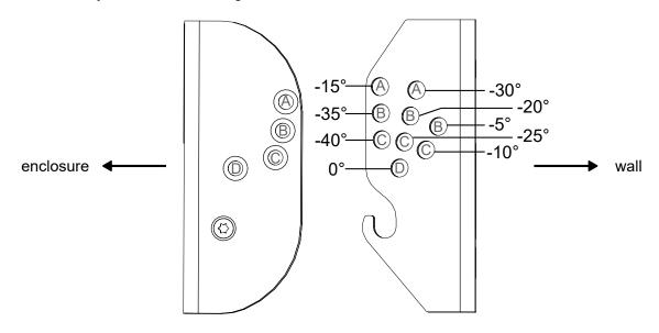
c) Drive the axis through the holes and secure it with the M4×16 Torx screw.
