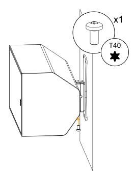
**7.** Rotate the assembly to adjust the azimuth angle.
