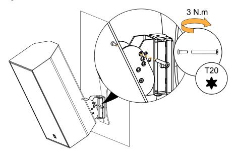
10. Rotate X8i to adjust the azimuth angle from -45 $^{\circ}$  to +45 $^{\circ}$ .
