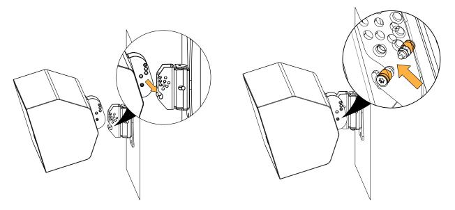
b) Rotate the assembly to select the site angle.
