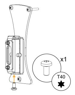
6. Remove the two placeholder screws in the middle of X8i.
