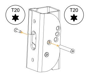
3. Assemble the TILT wall-mounting part with TILT-SUPPORT.
