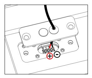
**5.** Secure the connector sealing plate to the enclosure.
