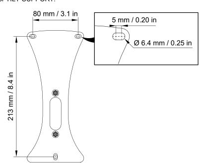
$\textbf{2.} \ \ \text{Assemble the wall-mounting plate and tapered spacers with TILT-SUPPORT}.$
