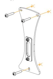
**4.** Remove the two placeholder screws at the bottom of X8i.
