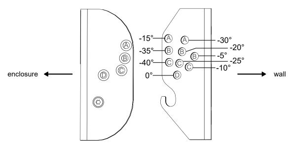
c) Drive the axis through the holes and secure it with the M4×16 Torx screw. Make sure that the assembly is stable.
