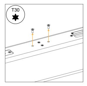
2. Secure CEILING-PENDANT to X8i. Use two M6×25 Torx screws.
