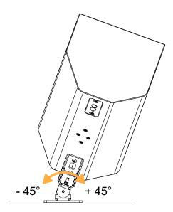
Tighten the M8×16 Torx screw. Apply a torque of 10 N.m.
