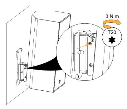
10. Rotate the assembly to adjust the azimuth angle from -45 $^{\circ}$  to +45 $^{\circ}$ .
