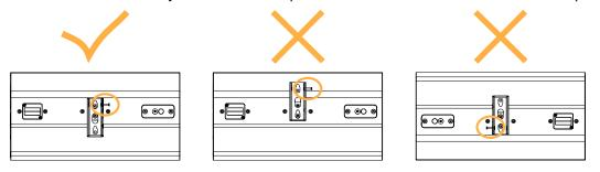
If the shank of the screwdriver collides with TILT40, use a screwdriver extension or an angled screwdriver to drive the screws.
