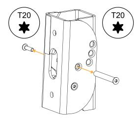
$\textbf{3.} \ \, \textbf{Assemble the TILT wall-mounting part with TILT-SUPPORT}.$
