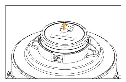
**2.** Remove the two screws securing the HF driver. Use the 3 mm hex bit.
