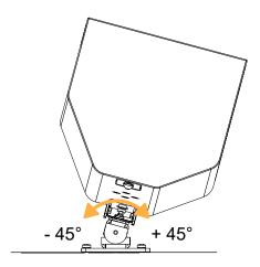
**11.** Tighten the M8×16 Torx screw. Apply a torque of 10 N.m. Make sure the assembly is stable.
