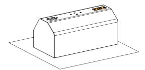
• For GROUND35 (35° site angle): with the connector plate on the left.
