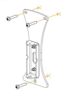
**4.** Disassemble the two TILT parts.
