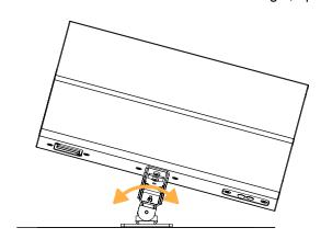
**11.** Tighten the M8×16 Torx screw. Apply a torque of 10 N.m.
