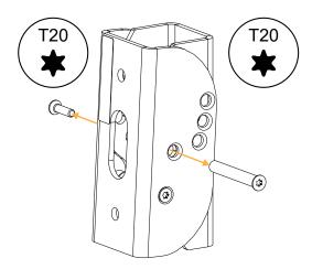
**5.** Assemble the PAN enclosure-mounting part with the TILT wall-mounting part. Use the two M6×25 Torx screws, M6 nuts and washers.
