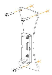
**4.** Disassemble the two TILT parts.
