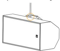
1. Choose the pickup point and secure X8i-HBAR to a truss clamp or to a threaded rod (maximum  $\emptyset$  10 mm / 0.39 in) using nuts.
