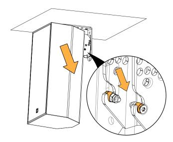
b) Rotate the assembly to select the site angle.
