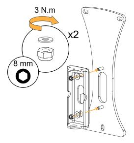
3. Secure TILT-SUPPORT and PAN to the wall.
