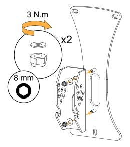
4. Secure TILT-SUPPORT and TILT to the wall.
