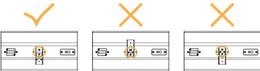
Make sure the rectangular washer is in the correct position.
