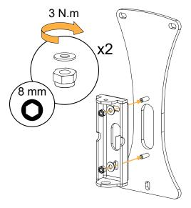
3. Secure TILT-SUPPORT and PAN to the wall.
