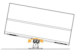
**13.** Tighten the M8×16 Torx screw. Apply a torque of 10 N.m. Make sure the assembly is stable.
