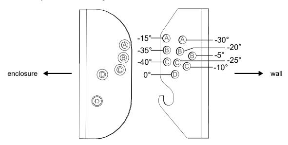
c) Drive the axis through the holes and secure it with the M4×16 Torx screw. Make sure the assembly is stable.
