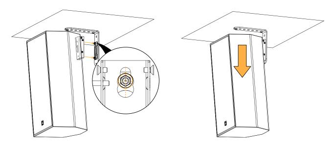
7. Tighten the safety screw and make sure the assembly is stable.
