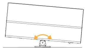
Tighten the M8 screw. Apply a torque of 10 N.m. Make sure the assembly is stable.
