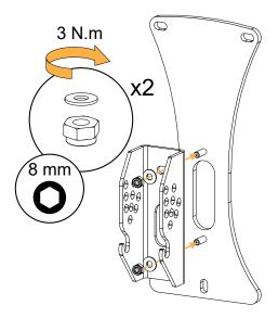
4. Secure TILT-SUPPORT and TILT to the wall.
