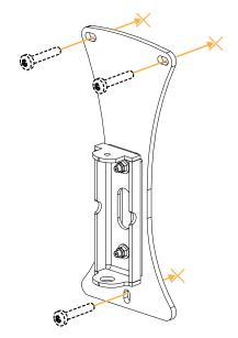
**4.** Assemble the wall-mounting plate and tapered spacers with PAN. Use two M5×20 Torx screws, two M5 washers, and two M5 nuts. The wall-mounting plate gasket is facing away from PAN.
