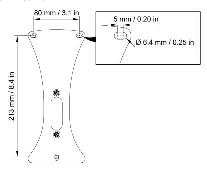
2. Assemble the PAN wall-mounting part with TILT-SUPPORT.
