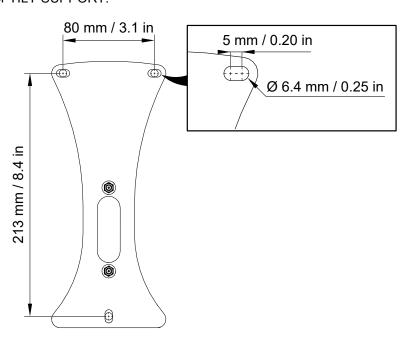
2. Assemble the PAN wall-mounting part with TILT-SUPPORT. Use the two M5 nuts and washers.
