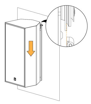
7. Tighten the safety screws on both sides and make sure the assembly is stable.
