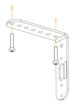
3. Assemble the wall-mounting plate and tapered spacers with VBAR.
