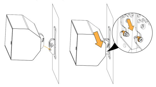
b) Rotate the assembly to select the site angle.
