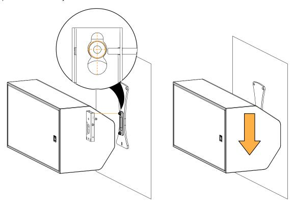
**9.** Tighten the safety screw and make sure the assembly is stable.
