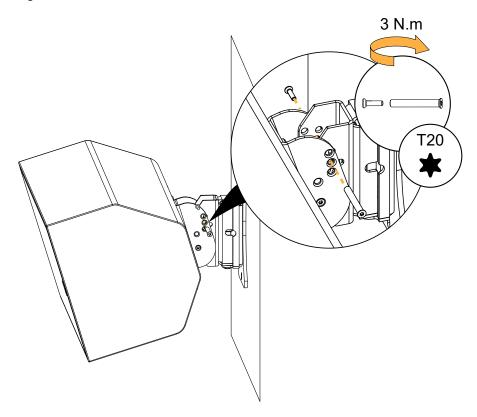
**10.** Rotate the assembly to adjust the azimuth angle.
