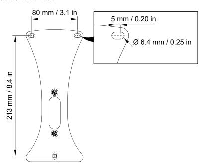
**2.** Assemble the wall-mounting plate and tapered spacers with TILT-SUPPORT.
