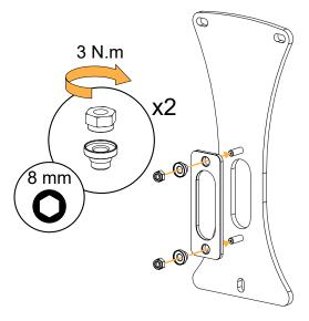
3. Secure TILT-SUPPORT and the wall-mounting plate to the wall.
