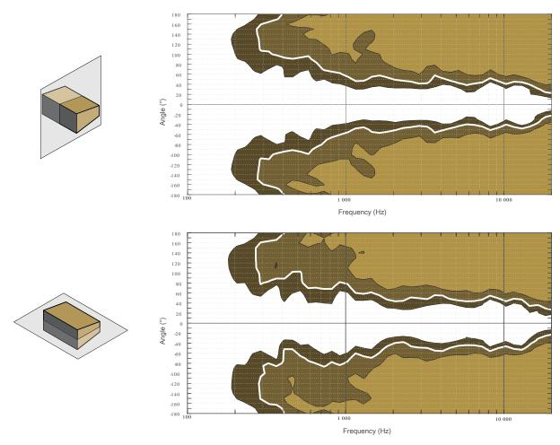
Dispersion angle diagram of a single X8i using lines of equal sound pressure at -3 dB, -6 dB, -12 dB.
