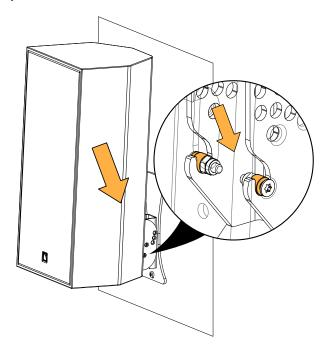
b) Rotate the assembly to select the site angle.
