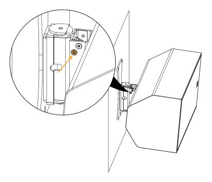
**12.** Rotate the assembly to adjust the azimuth angle.
