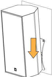
8. Tighten the safety screw and make sure the assembly is stable.
