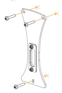
**4.** Remove the two placeholder screws in the middle of X8i.
