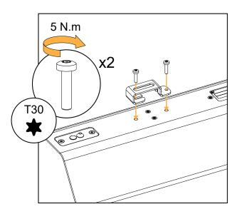
3. Fly X8i with a truss clamp or a threaded rod (maximum  $\emptyset$  12 mm / 0.47 in). Make sure the assembly is stable.
