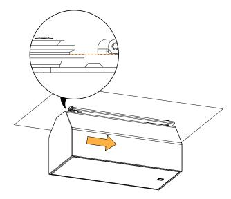
7. Tighten the safety screws on both sides and make sure the assembly is stable.
