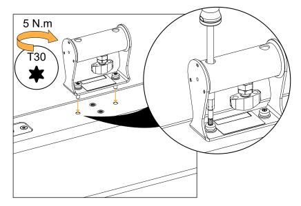
3. Mount the assembly on a  $\emptyset$  35 mm (1-3/8") pole.
