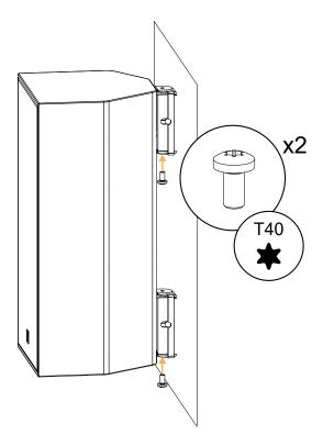
7. Rotate X8i to adjust the azimuth angle from -45 $^{\circ}$  to +45 $^{\circ}$ .
