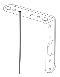
3. Remove the two top placeholder screws.
