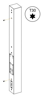
4. Mount the silent blocks to Soka with the two M6x35 Torx screws.
