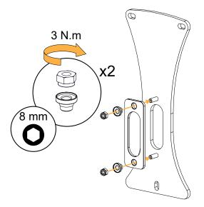
**4.** Secure TILT-SUPPORT and the wall-mounting plate to the wall. Run the speaker cable through the assembly.
