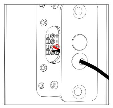
Secure the connector sealing plate to the enclosure. Apply a torque of 3 N.m.
