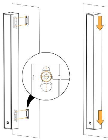
7. Tighten the two safety screws and make sure the assembly is stable.
