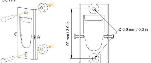
3. Remove the two placeholder screws from the back of Soka.
