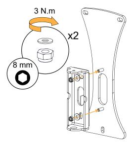
**4.** Secure TILT-SUPPORT and PAN to the wall. Run the speaker cable through the assembly.
