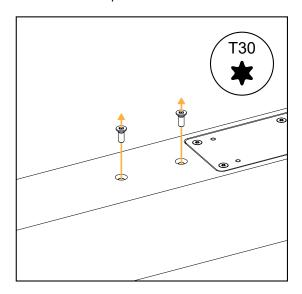
2. Secure POLE to Soka with the two captive screws.
