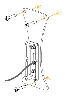
5. Assemble the wall-mounting plate and tapered spacers with PAN.
