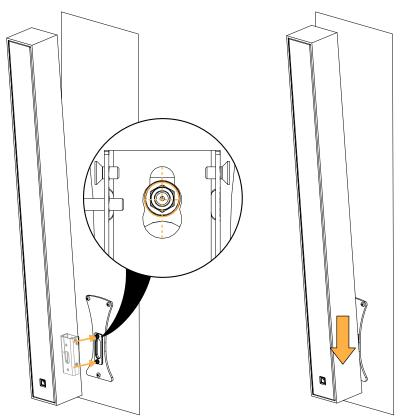
7. Tighten the safety screw and make sure the assembly is stable.
