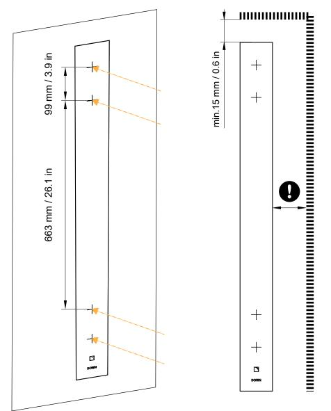
2. Secure the surface-mounting plate on the wall, using the four spacers.
