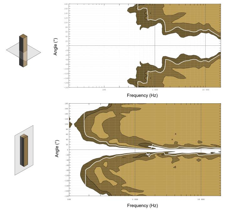
Dispersion angle diagram of a single enclosure, using lines of equal sound pressure at -3 dB, -6 dB, -12 dB.
