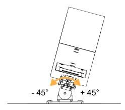
Tighten the M8x16 Torx screw. Apply a torque of 10 N.m. Make sure the assembly is stable.
