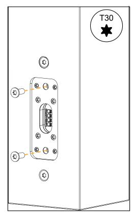
2. Insert the cable through the cable gland.
