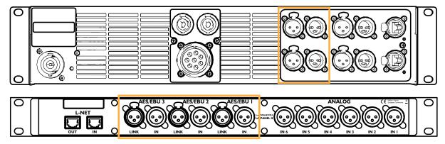
The IN connectors of the front of LA-PANEL II are cabled to an AES/EBU IN connectors on the LA12X amplified controllers using the appropriate IN XLR cable. The AES/EBU LINK connectors on the LA12X amplified controllers are cabled to the LINK connectors of the LA-PANEL II using the appropriate LINK XLR cable.
