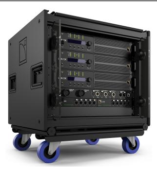
LA-RAK II AVB is a flyable touring rack offering twelve channels of high power amplification in a 9U frame. It is equipped with three LA12X amplified controllers, two LS10 AVB switches, two panels for mains power and signal distribution and a blank panel. All devices are internally prewired for audio, control and power to offer a plug-and-play solution with seamless networked audio redundancy based on the Milan protocol.
