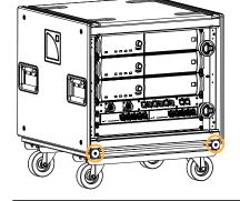
bottom rails are not damaged screws are tightened
