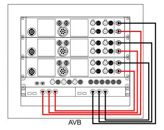
Different cabling schemes are available in Analog mode. Refer to Analog audio cabling (p.46) for more cabling options.
