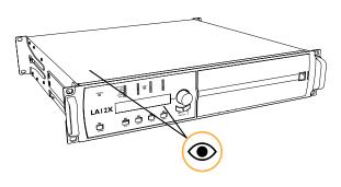
chassis, Lexan plate, LCD screen, and LEDs are not damaged
