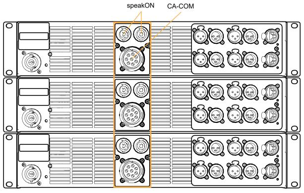
Consider supporting the cables connected to the 8-point outputs to reduce mechanical stress on the LA12X chassis, in particular when flying LA-RAK II AVB.
