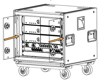
3. Insert and lock the ball-locking pins through each door's safety hole to secure the doors.
