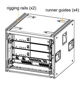
Connection with other LA-RAK II AVB or rigging elements is ensured by two coupling bars with spring-loaded safety.
