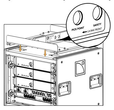
2. Disconnect LA-RAK II AVB from the dolly board by removing the coupling bars.
