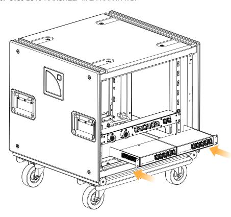
**4.** Secure LS10-RAKSHELF to the front face of the rack using the two spacers, the M6×20 screws, and the washers. Secure the 1U blank panel under the switch.
