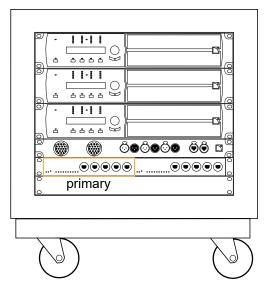
By convention, black Ethernet cables are used to connect the primary LS10 to the first port of each LA12X using ports 8, 9 and 10 at the back of LS10. Similarly, the right LS10 (as viewed from the front of LA-RAK II AVB) pertains to the Secondary network. By convention, red Ethernet cables are used to connect it to the second port of each LA12X using ports 8, 9 and 10 at the back of LS10.
