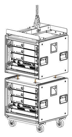
7. Disconnect LA-RAK II AVB from the dolly board by removing the coupling bars.
