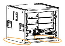
screws are tightened stacking runners are present and not damaged
