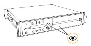
encoder wheel, and grill and foam filter are present and not damaged
