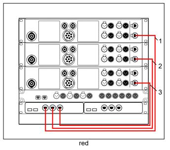
Six Ethernet etherCON cables are connected to LA12X. Red cables and black cables are used to distinguish the networks. Three first cables create a Primary network (black). Three other cables create a Secondary network (red).
