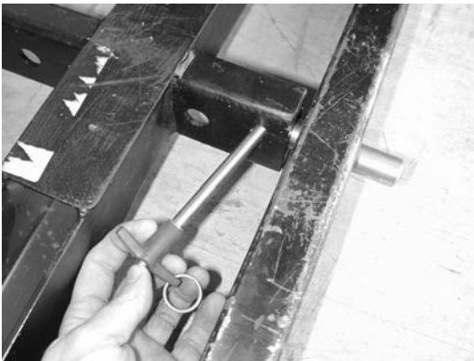
(v) Use dV-PIN81 to secure locator pin
