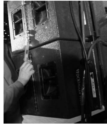
(viii) Connect ANGLE straps on bottom V-DOSC
