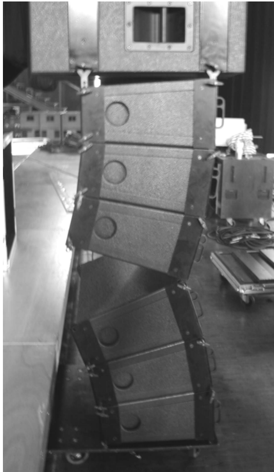
Figure 88: Rigging dV-DOSC under dV-SUB (larger configuration – procedure 2)
