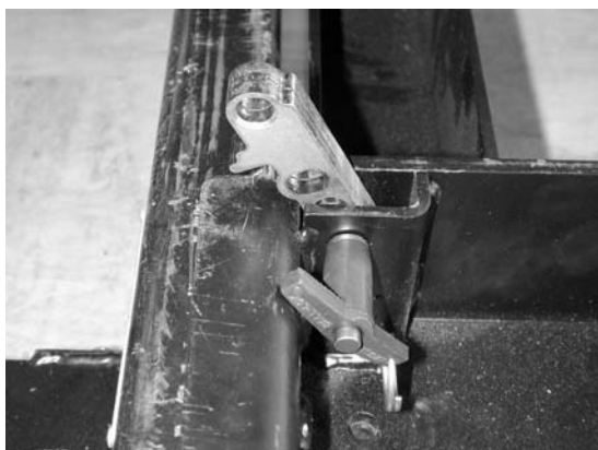
(ix) dV-ANGLE pre-attached in the 3.75 degree position
