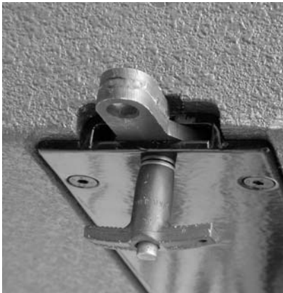
(i) dV-ANGLEDSD pre-attached - note that the stacked hole position has been selected and the "fat" part of the angle bar is oriented towards the center
