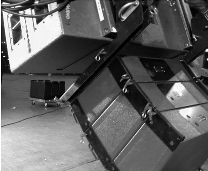
(ix) Raise the ARRAY - note the gap
