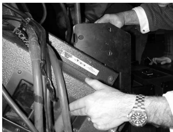
(iv) Align rotating leg with holes on dV-DOWN
