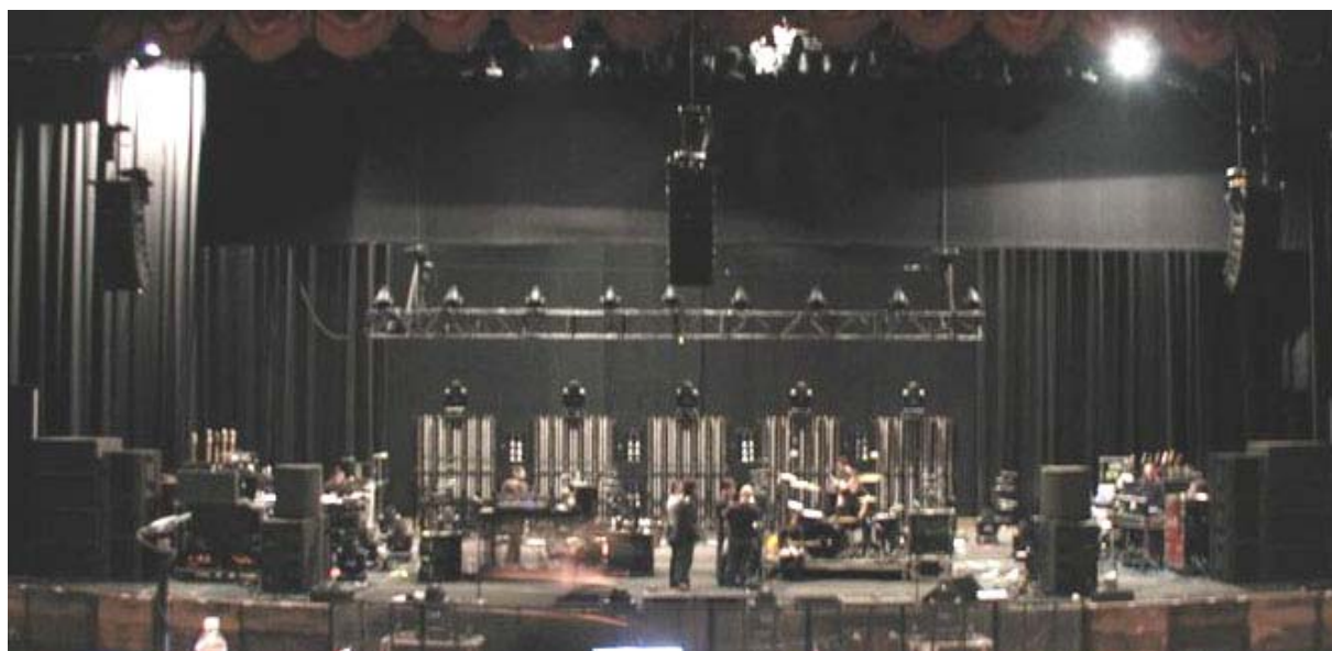
Figure 61: LCR Configuration: 3 x 9 dV-DOSC, 4+4 SB218, 3+3 dV-SUB FOH system; 2+2 ARCS, 2+2 SB218 sidefill monitor system (Nine Inch Nails 2005 US tour, sound designers: F. Bernard; M. Prowda)
