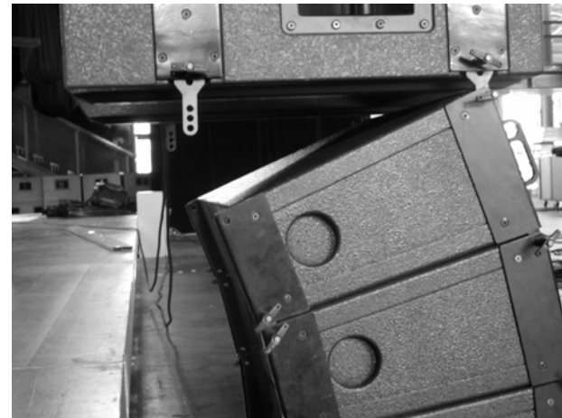
(iv) dV-DOSC front point attachment using dV-ANGLEDSD. The array is raised and rear points attached using dV-ANGLEDSDP
