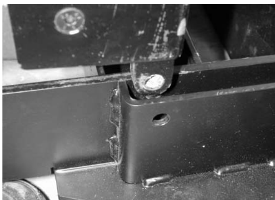
(x) Front rigging tabs mate with locator slots on dV-BUMP
