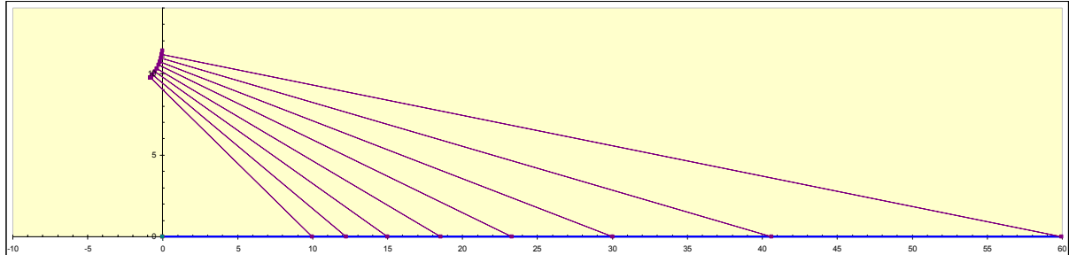
Figure 46 (a): Cutview showing non-constant enclosure site angle impact spacing for an 8 enclosure constant curvature dV-DOSC array (4.5 degrees between all enclosures)
