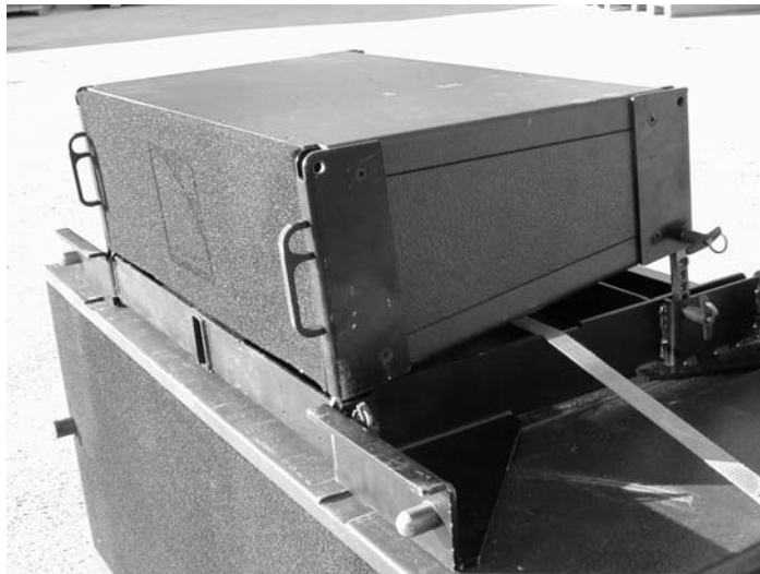
(vii) Bottom dV-DOSC mounted, attached using dV-PIN25
