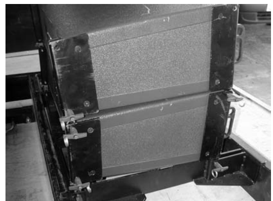
(xv) Pin front points first, rear points last using dV-PIN25
