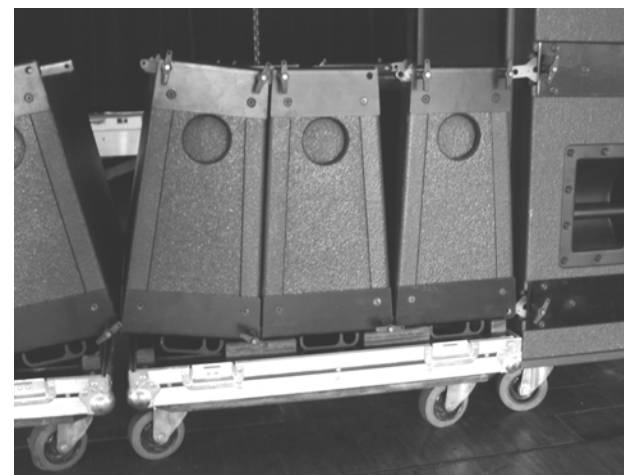
(vi) All dV-DOSC attached at front, in blocks of 3 at the rear (except for dV-DOSC #1 to #2)
