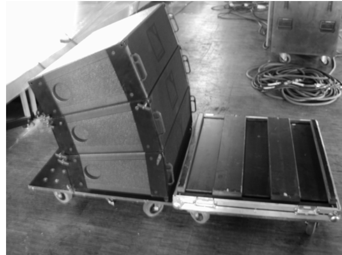
(ii) Flip dV-DOSC onto dV-SUB dolleys to position under the dV-SUB array
