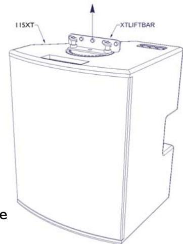
L-ACOUSTICS has engineered the I15XT and its rigging accessories using state of the art modeling and calculation software. The ETRI15XT, the CPLI15XT and the XTLIFTBAR rigging accessory were also destructively tested to validate the final design using a pulling bench equipped with laboratory calibrated measuring cells.
