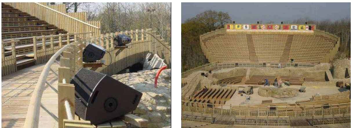
FIGURE 24: INSTALLATION DISTRIBUEE EN I 12XT (PUY DU FOU, FRANCE)
